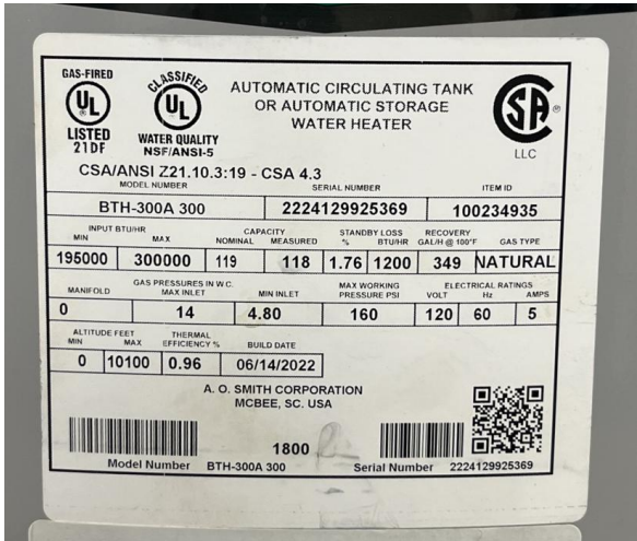
Figure 8: Domestic water heater label
