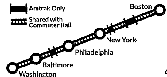
Shared Tracks on the Northeast Corridor main line
